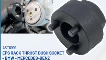
AST6199 specialist socket displays a 24mm hex drive and enables the adjustment or removal / installation of the thrust bush, whilst the rack is still in position on the vehicle.
